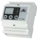
**C.MG module** - allows for additional heating system control (i.g. floor heating). Using additional C.MG modules ensures control over mixing valves, that reduces heating water temperature for each circulation system. Up to 24 C.MG modules may be connected to the C.PS unit.
